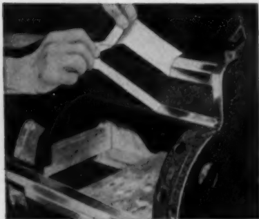
2. MASKING TAPES have flexible creped backings to allow them to fit curves and irregular surfaces easily. Above, High Heat Masking Tape No. 214 protects chrome on cash register; withstands temperatures up to 375°F. for several bakes; leaves no residue.
